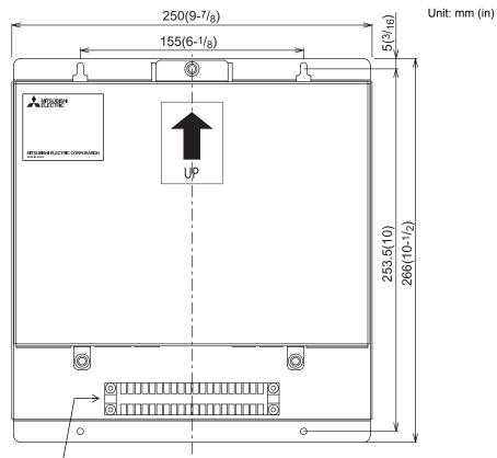
Terminal block (to be used in the future when functions of the BAC-HD150 are upgraded.)
